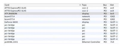
MAC System Profiler with 2 PCIe to PCI Expansion Systems Installed in a "Fan-Out Configuration.
